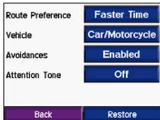
**Route Preference**—select a preference for calculating your route. Select **Faster Time** to calculate routes that are faster to drive but can be longer in distance. Select **Shorter Distance** to calculate routes that are shorter in distance but can take more time to drive.
